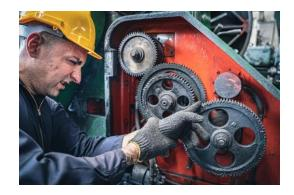
Other forms of hazardous energy that can cause injury if not properly discharged include elevated machine members, rotating flywheels, hydraulic systems, air gas, steam, and water pressure. Refer to your District's LOTO policy for equipment specific deenergization steps.
